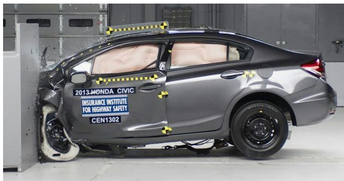
Figure 2: Frontal crash test required by FMVSS 208 [1].
